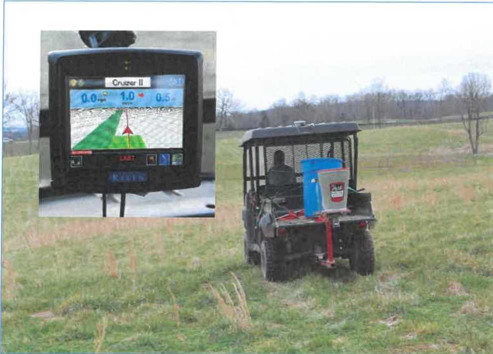
Figure 2. Frost seeding is accomplished by broadcasting clover seed onto closely grazed pastures in late winter or early spring. Using GPS guidance helps operators maintain equal spacing between passes and consistent speed (inset picture). (Photos by Chris Teutsch)
