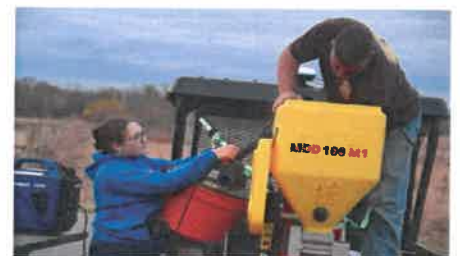
Figure 3. Sweeping remaining seed out to determine the seeding rate by difference.
