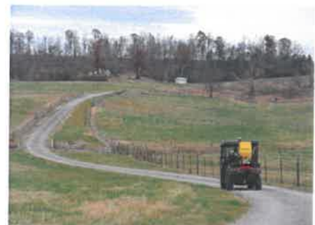
Figure 2. A UTV with the APV seeder mounted in the bed was driven on a paved course that was 1,000 ft in length.
